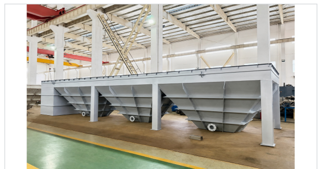
Actual-project hopper-bottom process tank | integrated supports and discharge zones
